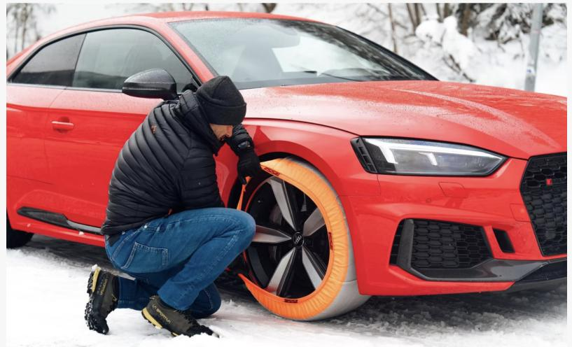
ISSE, the world leader in textile traction devices, has introduced an essential emergency solution for North American drivers: tire socks that prevent slipping and sliding on ice or snow
