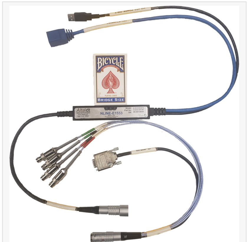
NLINE-E1553 Real-Time, In-Line 1553 Ethernet Converter. Industry's First Full Featured In-Line 1553 Product.
