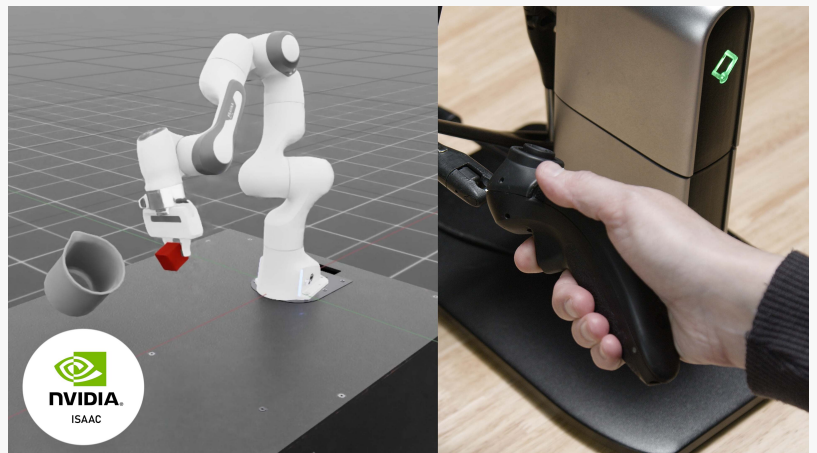
Haply's Inverse3 device controlling a Franka FR3 robotic arm inside NVIDIA Isaac Sim
