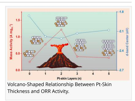
skin that delivers the fastest oxygen reduction, exceptional durability, and record-high activity. This work not only pinpoints why this configuration excels but also establishes a roadmap for constructing more efficient, low-Pt catalysts for clean energy systems.
