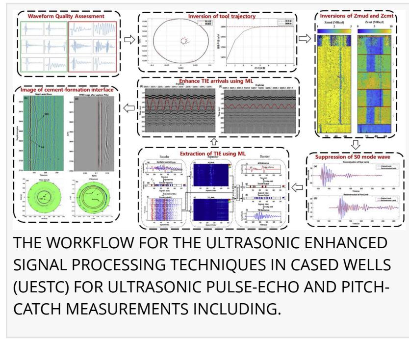
Ensuring the integrity of wells is fundamental to safe oil and gas production, geothermal energy development, and geological carbon storage. At the heart of well integrity lies cement bonding, which isolates subsurface formations and prevents hazardous fluid migration. Against this backdrop, a team of researchers from China conducted a comprehensive review of recent advancements in [cement bond quality assessment](#) based on ultrasonic measurements.
