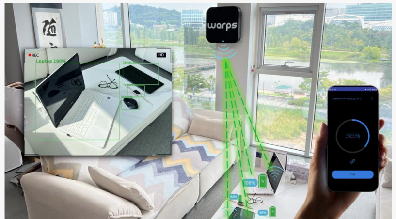
An example image showing AI tracking and beamforming-based wireless power transfer delivering RF energy to multiple devices
