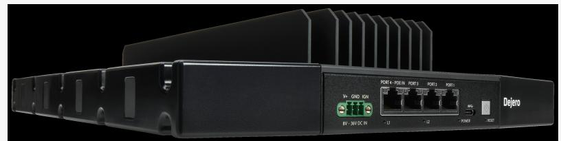
Integrated GPS/GNSS, PoE power, and packet-level network optimization in a ruggedized design (-40°C to 70°C / -40°F to 158°F).
