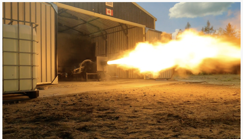
NordSpace - Engine Test of 3D Printed Hadfield Engine
