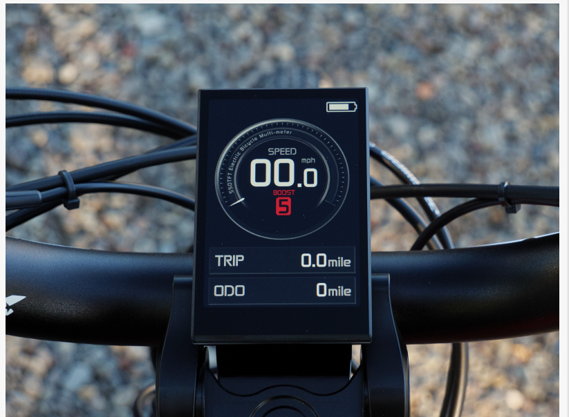
Handlebar-mounted color display on the Optibike G2 Loki showing speed, boost level, and trip information.
