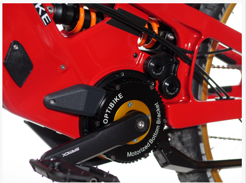
Close-up view of the Optibike G2 Loki motorized bottom bracket and drivetrain assembly.
