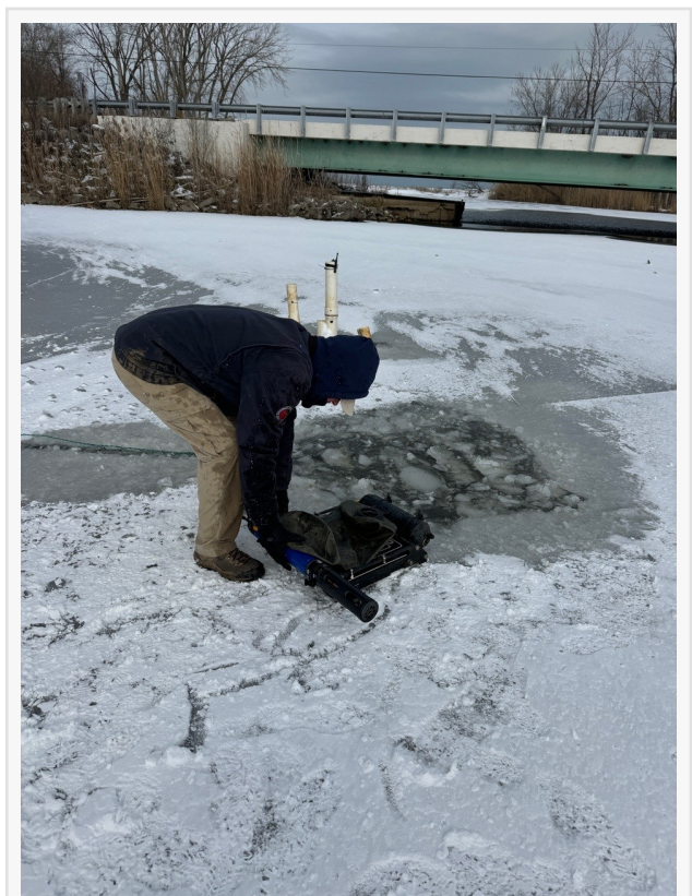
EM-2Q allows wireless through-ice monitoring
