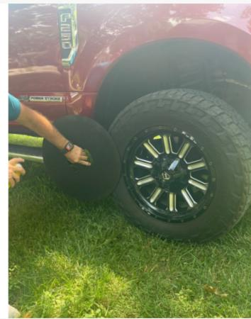
fully cover the wheel face while leaving the tire exposed for cleaning. The shield includes a first side, a second side, and a surrounding sidewall, with the first and second sides arranged in parallel to maintain a low-profile geometry. This flat configuration allows the shield to remain stable when placed against the wheel or temporarily set on the ground.
