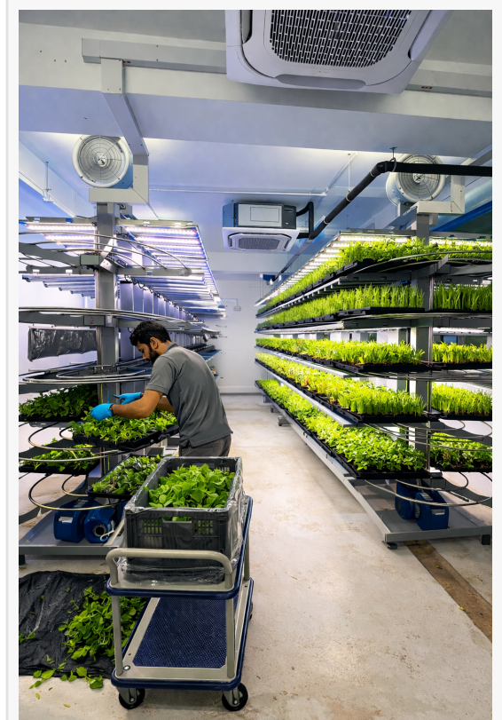
The BK Conveyor Culture (BKCC) vertical farming system in operation, designed to improve labor efficiency through horizontally revolving trays.
