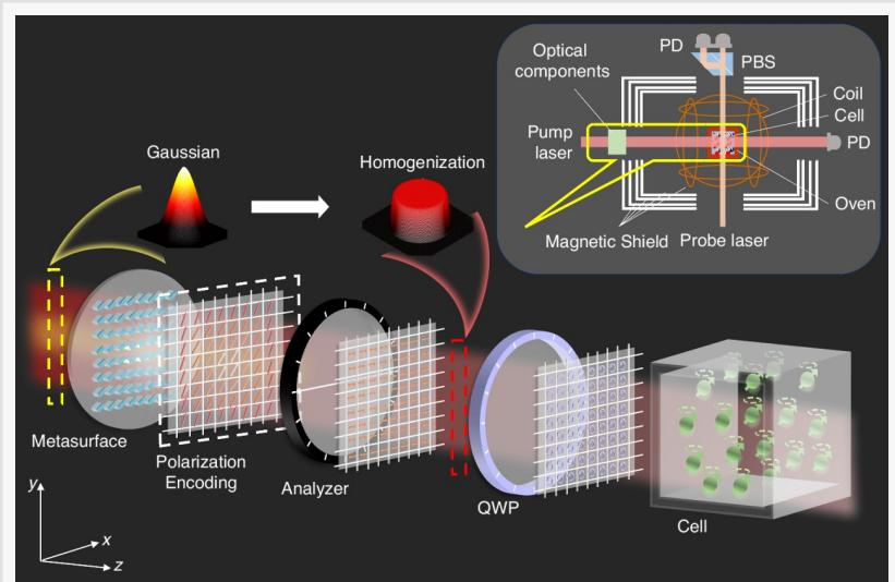
Schematic diagram of the beam homogenization method based on polarization-encoded metasurface.
