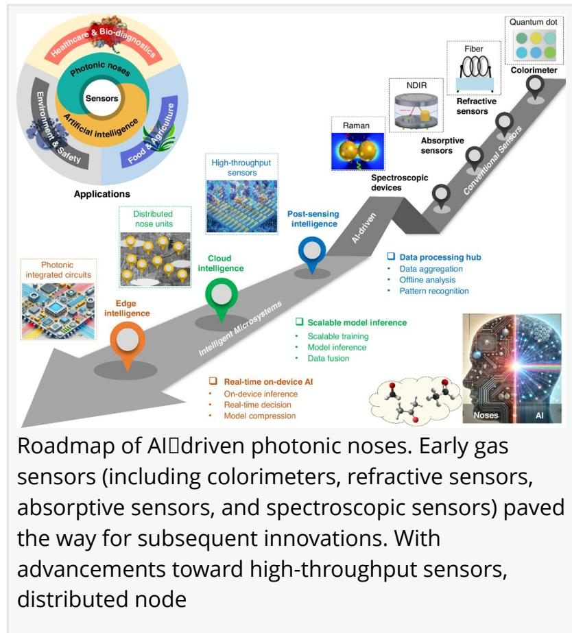
Roadmap of AI-driven photonic noses. Early gas sensors (including colorimeters, refractive sensors, absorptive sensors, and spectroscopic sensors) paved the way for subsequent innovations. With advancements toward high-throughput sensors, distributed node
