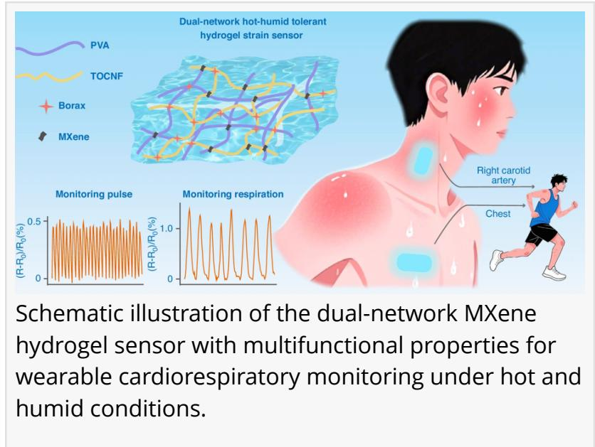
The sensor is built from a dual-network hydrogel composed of polyvinyl alcohol and oxidized cellulose nanofibers, reinforced with conductive MXene nanosheets and dynamic borate crosslinks. This architecture provides high stretchability—up to 800% strain—while preserving stable electrical signal transmission. The optimized hydrogel exhibits a gauge factor of 7.79, allowing it to detect subtle skin deformations associated with pulse waves and chest movements during breathing.
