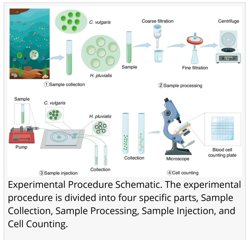
Experimental Procedure Schematic. The experimental procedure is divided into four specific parts, Sample Collection, Sample Processing, Sample Injection, and Cell Counting.
