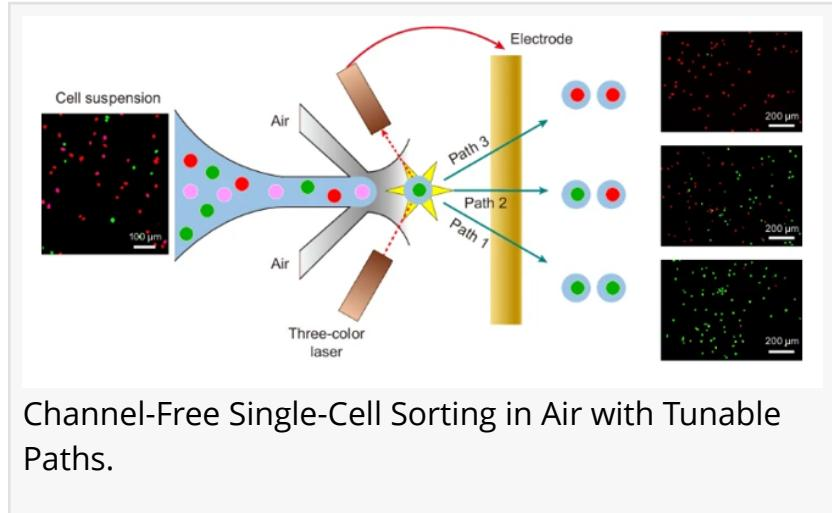
sorting paths in real time. This tunable ejection replaces fixed channel geometries and allows sorting routes to be reconfigured during operation.
