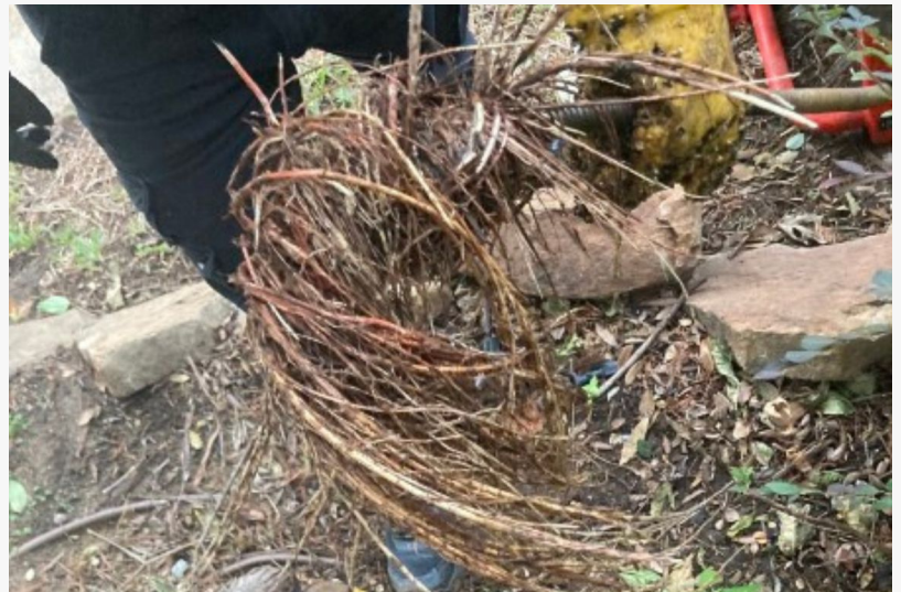
This massive root intrusion was pulled from a Dallas, TX home sewer line.
