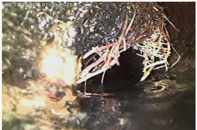
Sewer camera footage of intrusive tree roots causing a blockage.
