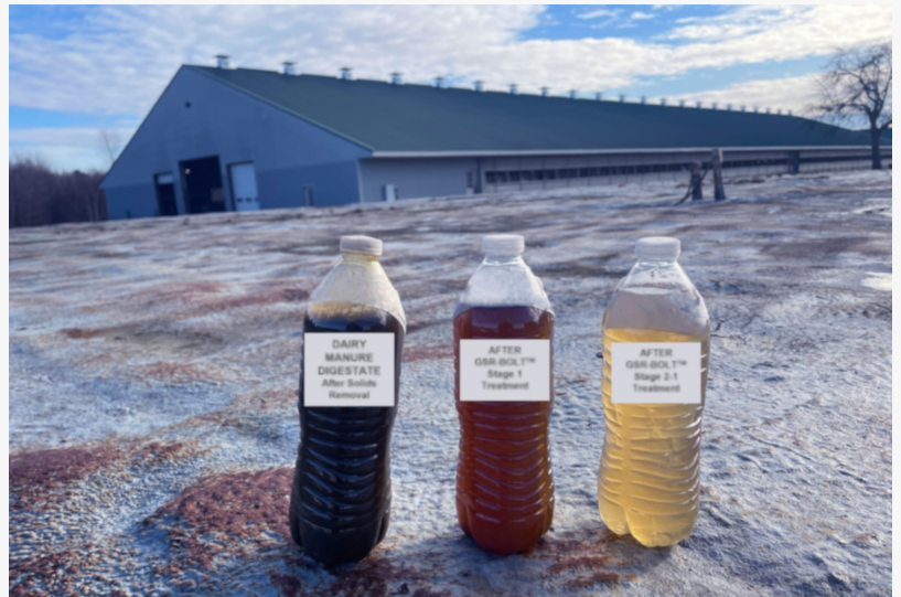
Manure-derived liquid effluent before treatment and after nutrient recovery treatment. (Courtesy of GSR Solutions)
