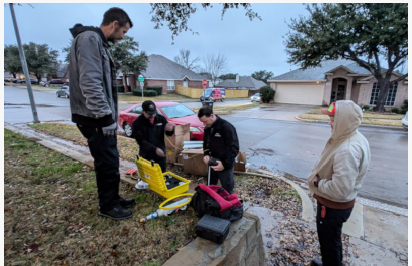
Electronic leak detection requires no digging or property damage to locate sewer leaks.
