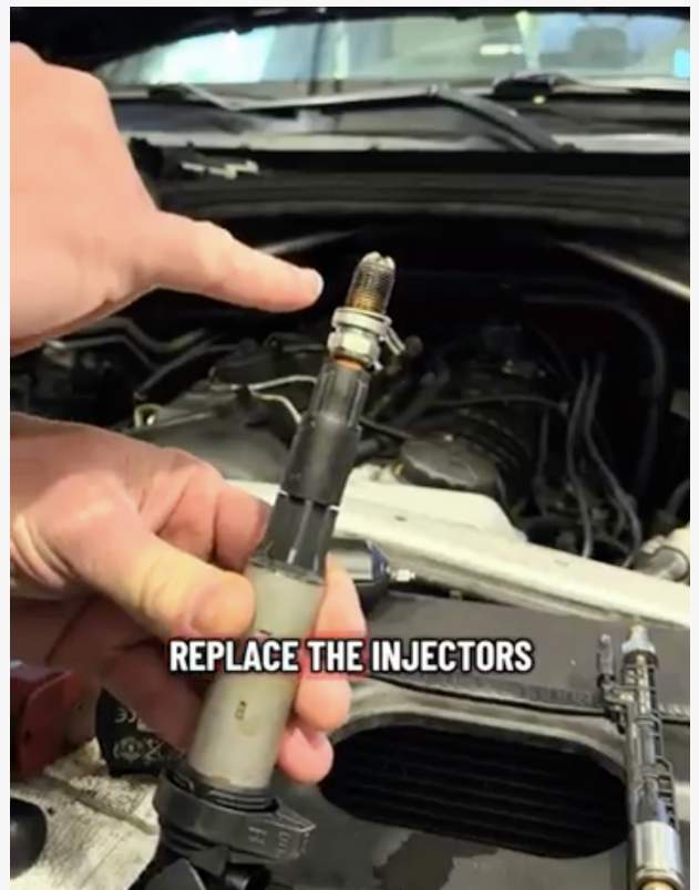
BMW X5 Spark Plugs with Carbon Buildup causing engine misfire codes.
