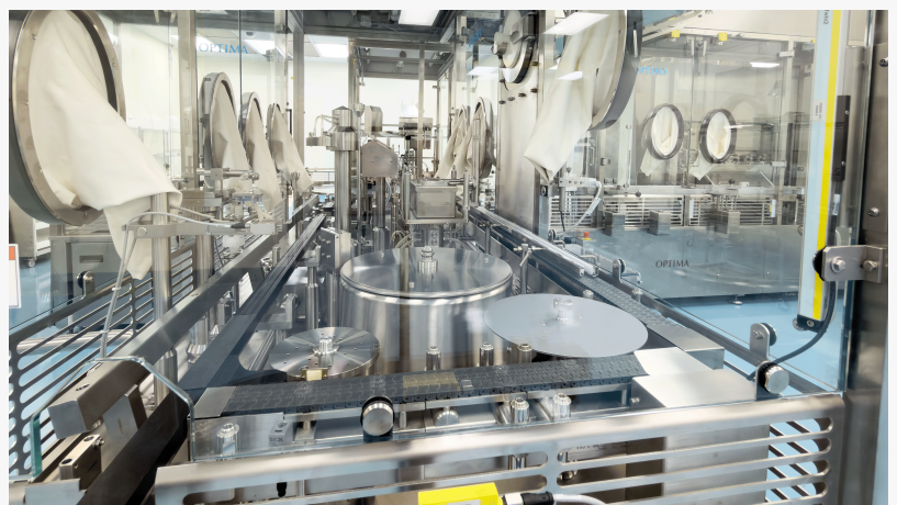
Automated Optima fill-finish line at BioTechnique, designed for high-precision vial filling with direct transfer into lyophilization.
