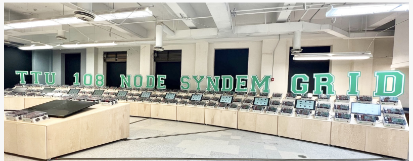
Autonomous power system with 108 physical power electronic converters
