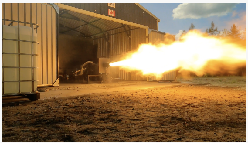
NordSpace's Darkhorse Engine Test Cell Firing the Company's 3D Printed Hadfield Engine
