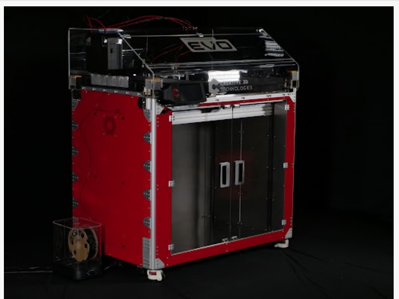
Creative 3D Technologies' EVO "Factory In A Box"
