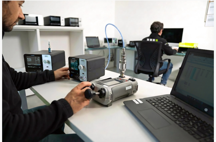
Use of ForTest leak tester in metrology laboratory
