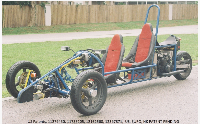
Three wheel motor vehicle. Two wheels in front. Drives like a car, leans like a sport bike.
