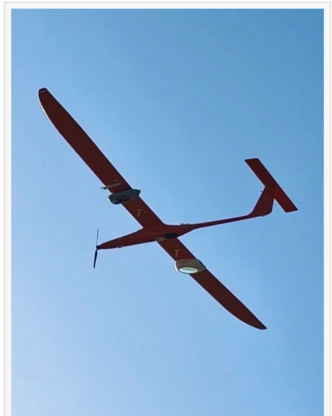
Kraus Hamdani Aerospace UAS in flight with attached PowerLight Technologies wireless power beaming receiver at Poinsett Electronic Combat Range
