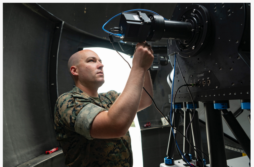
Naval Postgraduate School (NPS) graduate student U.S. Marine Corps Capt. Chris Henderson is using the NPS Mobile CubeSat Command and Control network and telescope to communicate with CubeSats using optical methods to transmit data.
