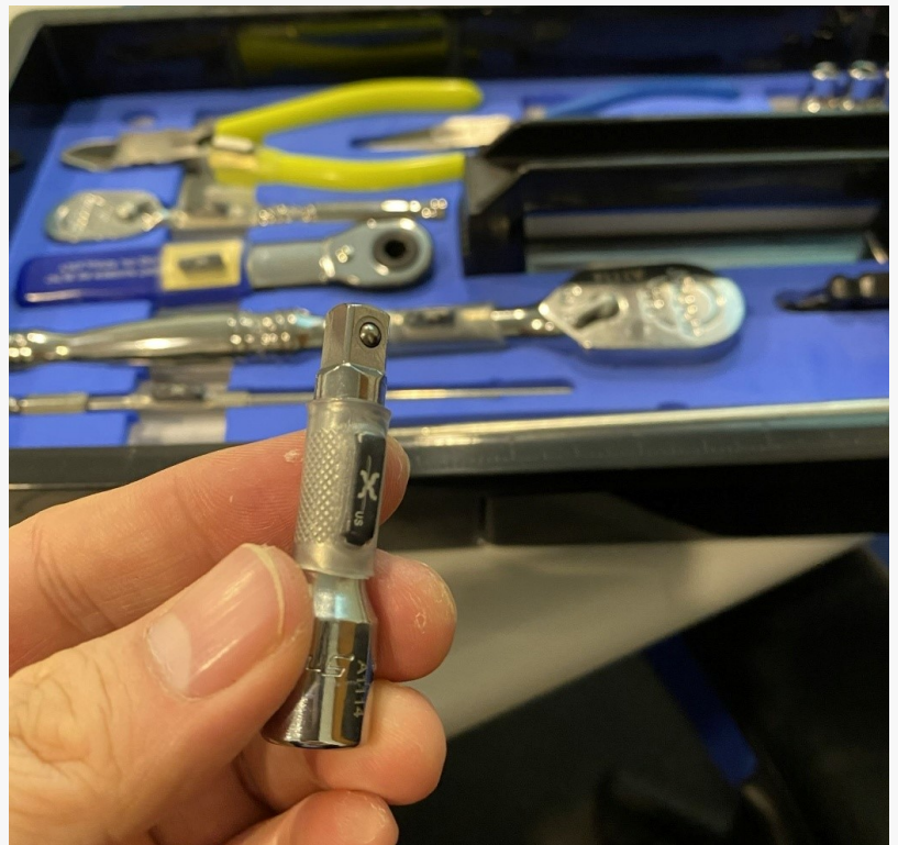
Xerafy RAIN RFID Tag XS Dash on the Small Tools
