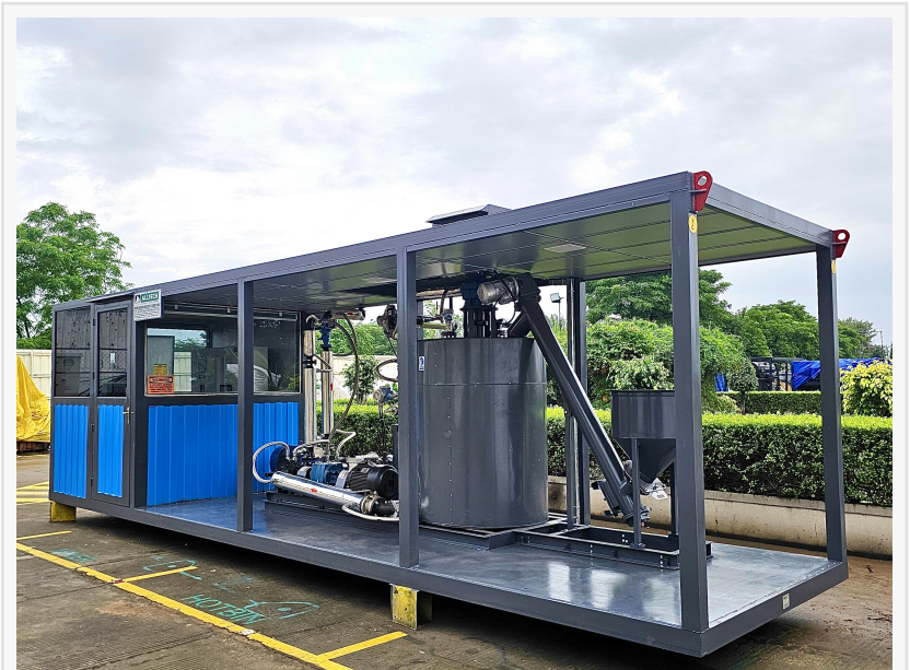
PMB / CRMB Plant
