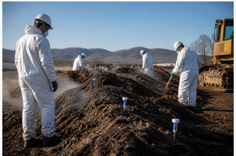
Field teams monitor mortality composting operations using real-time temperature sensors to ensure safety and performance.
