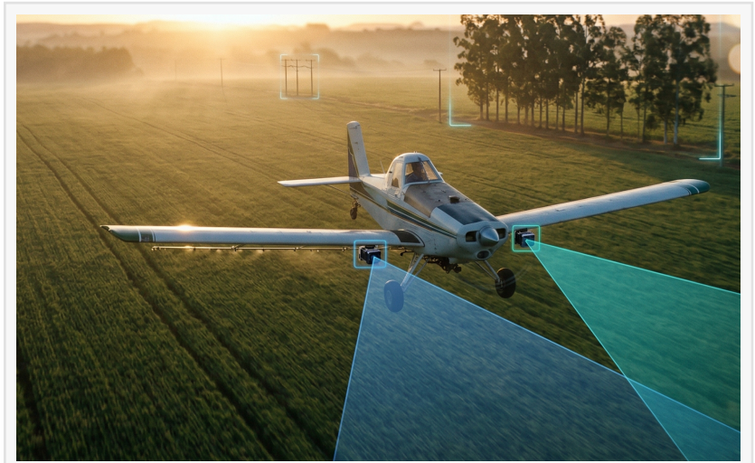
NODAR's FlightView brings automotive-proven 3D sensing to aviation, delivering real-time obstacle detection at ranges up to 1,000 m.
