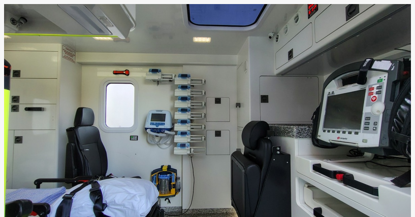
Inside Bryan Morgan Care's Intensive Care Ambulance, equipped for ventilated and ICU-level patient transport.
