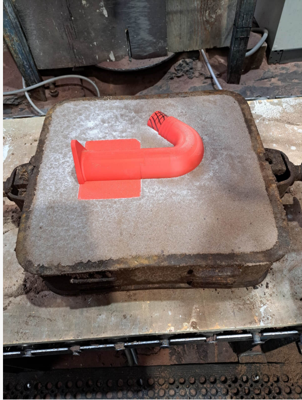
3D-printed pattern assembled ready for moulding
