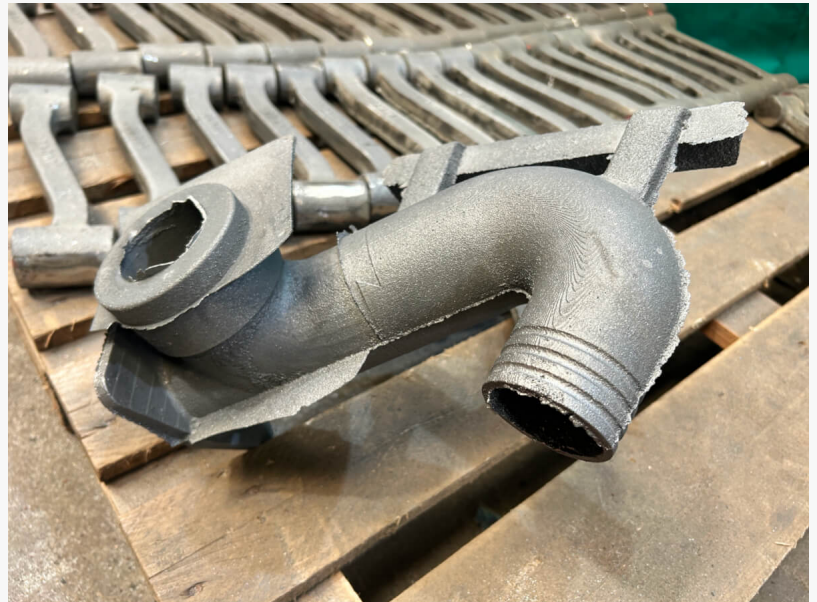
As-cast swan-neck component prior to finishing
