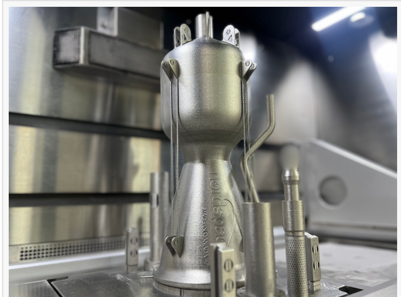
NordSpace – 3D Printed Hadfield Mk III Engine Produced at the Company's Advanced Manufacturing for Aerospace Lab (AMA Lab)
