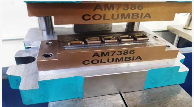
Embossing Plates Installed
