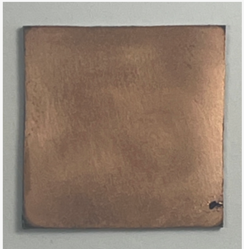
Copper film after curing in air
