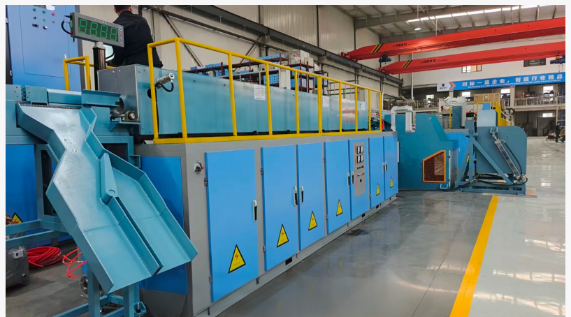
steel billet induction heating furnace-billet heating furnace with induction-copper billet heating system
