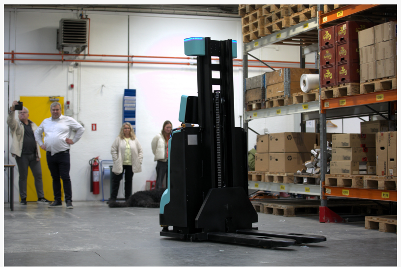
The J1600 self-driving pallet jack from The Mobile Robot Company during a demo day event
