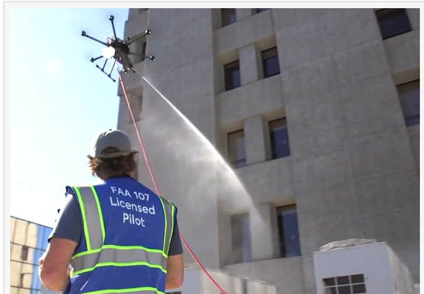
Aqua Drone Exterior Cleaning
