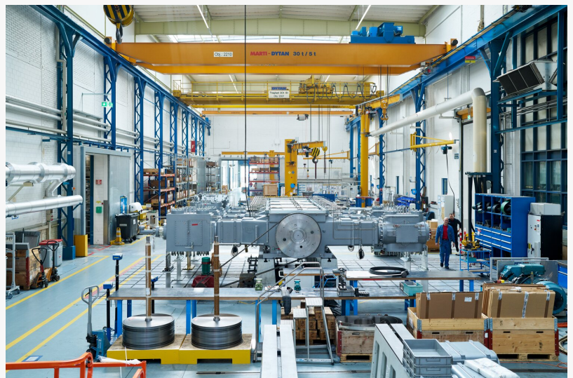
Assembly of a process gas compressor in Winterthur, Switzerland
