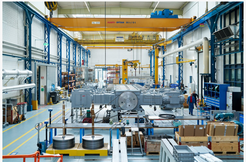
Montage eines Process Gas Compressors in Winterthur, Switzerland
