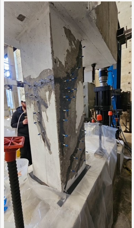
Purdue University Carbon Fiber Crack Repairs Test
