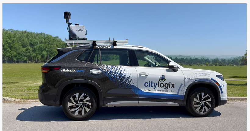
Citylogix's new VW survey vehicle, equipped with NIRA Dynamics' Tire Grip Indicator (TGI), captures IRI data on every survey pass.
