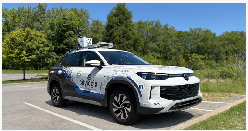
Front view of Citylogix's VW survey vehicle, equipped with NIRA Dynamics' Tire Grip Indicator (TGI).
