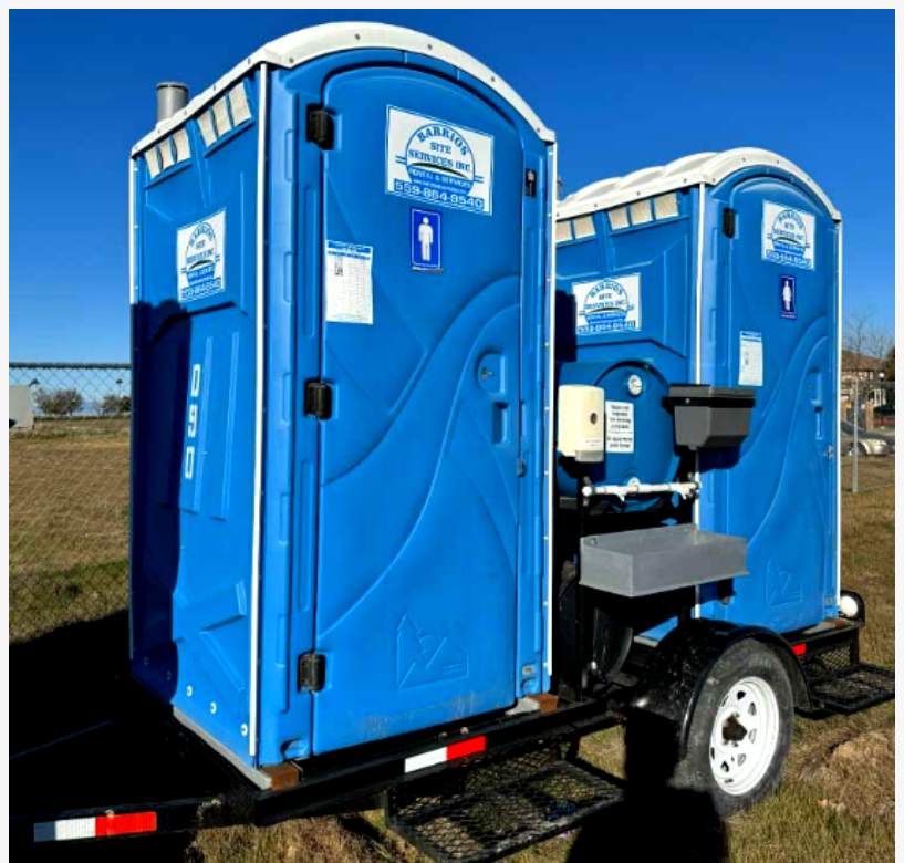
A towable unit featuring multiple portable toilets and integrated handwash stations, designed for mobility and efficiency on remote industrial or construction sites.
