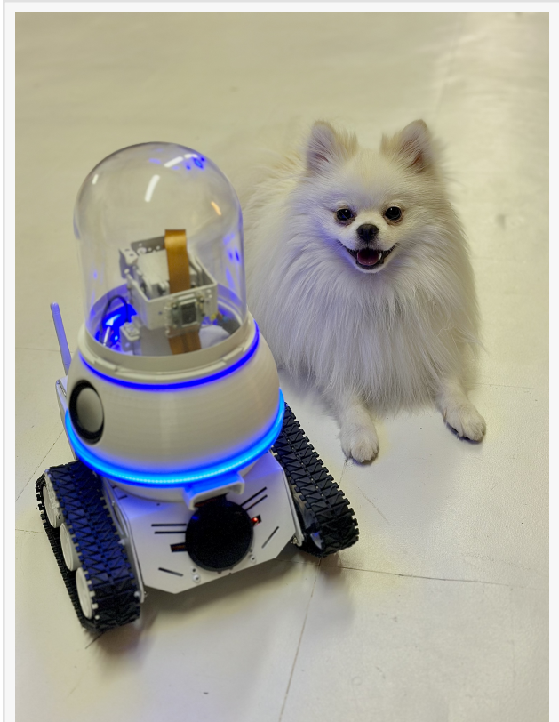
WIM-Z is an AI-powered home robot designed to monitor dogs, detect behaviors such as barking, and support positive reinforcement routines while owners are away.
