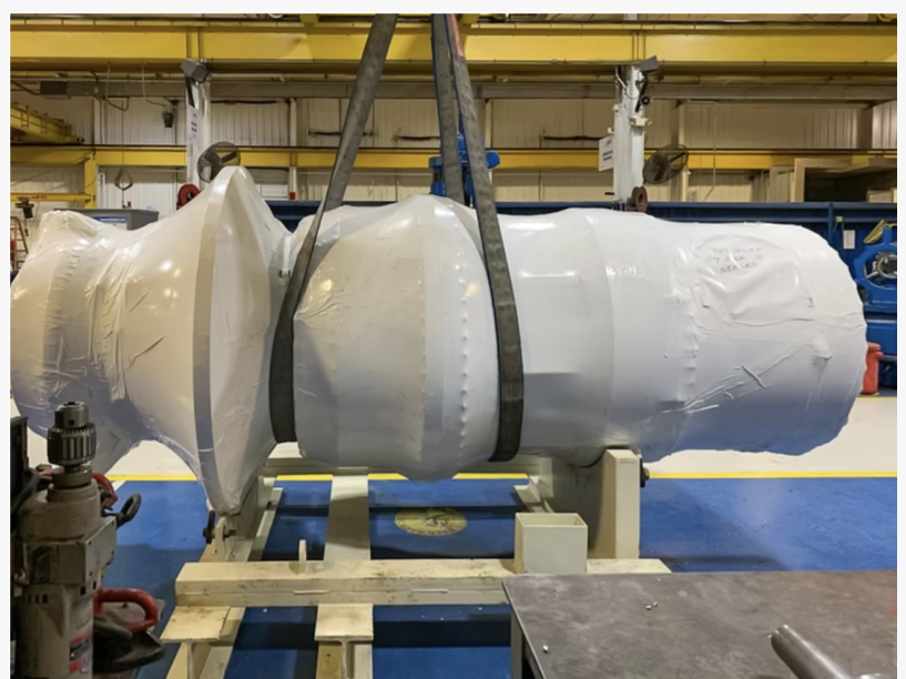
Industrial shrink wrap helps protect high-value equipment from moisture, UV exposure, contamination and shipping damage before transportation and storage.
