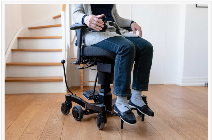
VELA mobility chair with Power Wheels, 360° maneuverability, and electric height adjustment
