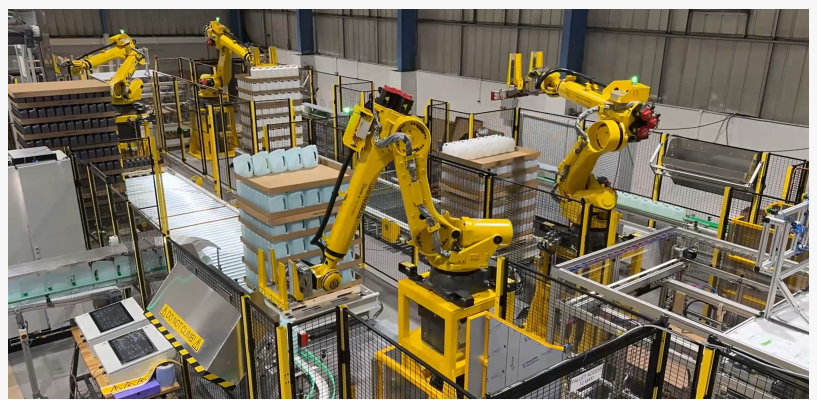
Robot pick and place and palletizing automation for container handling
